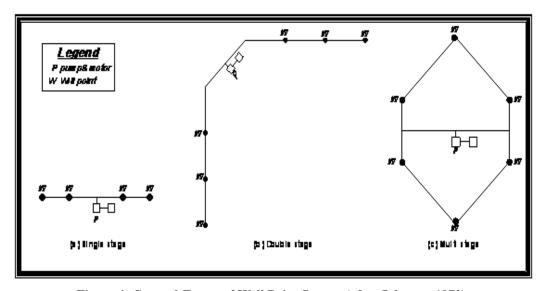
Figure 4: General Forms of Well Point System (after Johnson, 1972)
