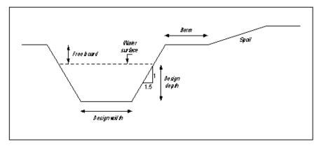
Figure 5: General Form of an Open Drain (after Luthin, 1978)
