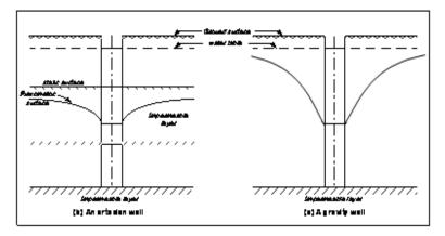
Figure 2: Vertical Drainage System (after Johnson, 1972)
