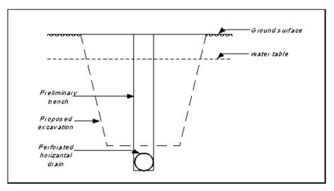
Figure 3: Horizontal Drainage System (After Johnson, 1972)
