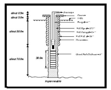
**Figure 6: Designed Well Section**
